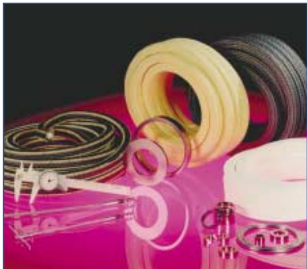
Figure 1. A few rolls of compression packing in the maintenance store will solve gland problems on most centrifugal and reciprocating pumps, and valves, at a site.
