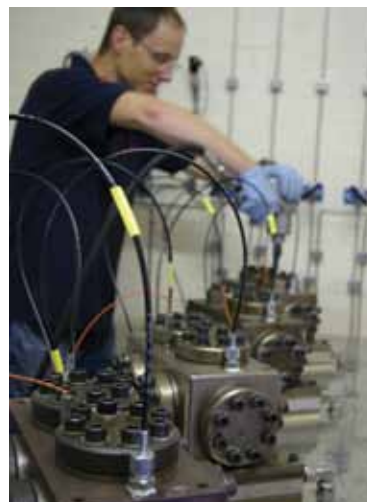
The James Walker Technology Centre incorporates a world-leading Rapid Gas Decompression testing facility.
