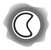
Distort seal in crescent fashion, and open out into housing recess with grooved side facing positive pressure. Carefully insert rod into position.
