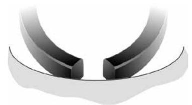
Fit the second ring, using the same technique, but ensure that the join is staggered about 90° from that of the first ring.
