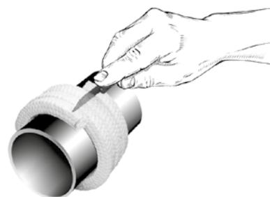
**i** A James Walker Compression Packing Cutter will simplify the ring cutting operation if scarf-split rings are to be used.
