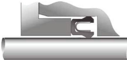
Expose the seal housing cavity by removing the gland follower or retaining plate. Insert the seal fully into the exposed cavity, with the seal's open face towards the system pressure.
