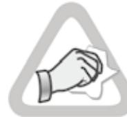
Remove old seal, and thoroughly clean the seal housing and lead-on/lead-in surfaces where seal must pass during installation.
