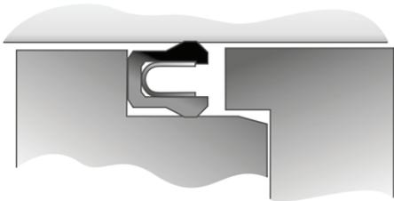
Ensure the seal is evenly seated around the entire circumference. Replace the gland follower or retaining plate, and carefully reassemble the equipment.
