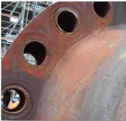
Photographs show nut galling of the flanges
