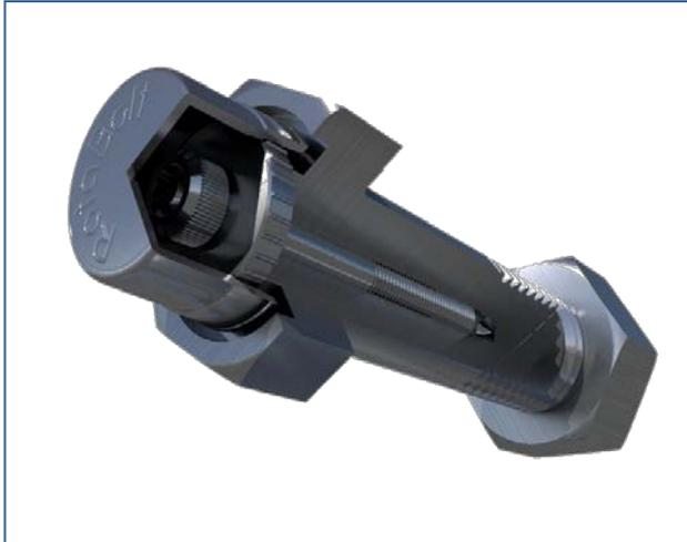
Each RotaBolt is individually 100% load test calibrated on installation, the rotating cap on the top of each bolt / stud locks when the correct tension is achieved and continues to provide a simple check of bolt tension in operation throughout the lifetime of the bolted joint. Should tension be subsequently lost for any reason, the cap will freely rotate.
