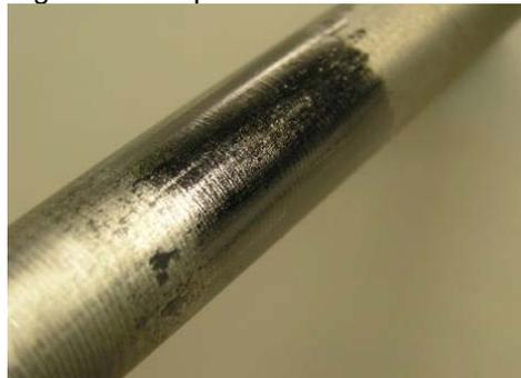
The images show as would be expected, a larger amount of material deposited on the rougher finished stems than smooth, to the point where a chromed finish is unable to hold any substantial packing deposit. The magnitudes of these differences are increased with 70MPa packing stress.
