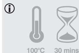
**i** If elastomeric sealing element cannot be stretched sufficiently, then warm it for about 30 minutes at 100°C in a conventional oven. Once warmed, follow the fitting guide instructions shown above. Follow local Health & Safety regulations for handling of hot items.
