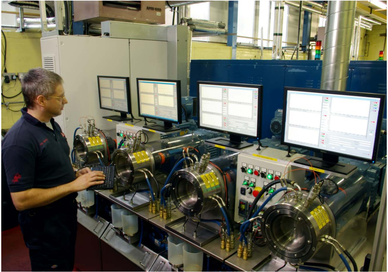
Fig 1: Fully computerised, multi-head test rig with continual data logging.
