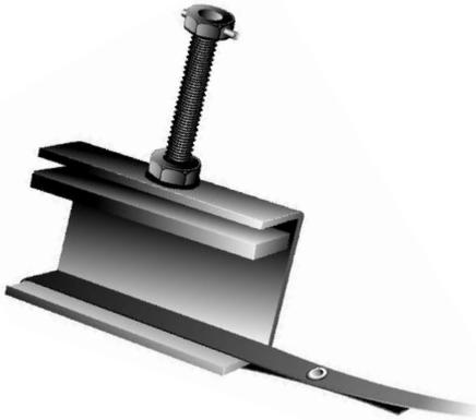
Hook one end of the *band* on to a clamp. Position clamp over a *jig* and tighten slightly to hold. Assemble second clamp with the other end of the *band*. Position the clamp over the second *jig* and slightly tighten to hold.
