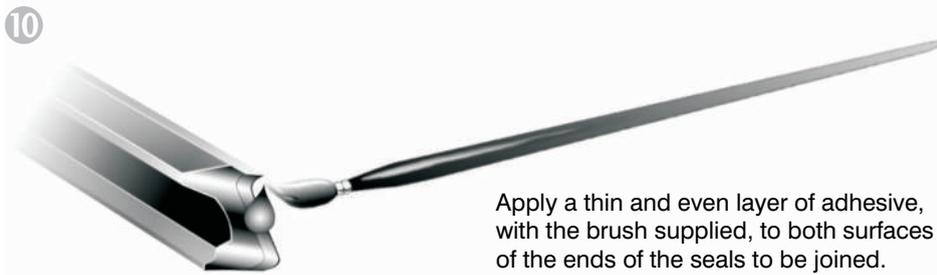
Apply a thin and even layer of adhesive, with the brush supplied, to both surfaces of the ends of the seals to be joined.
