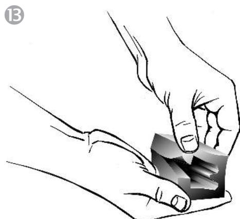
Allow the seal to cool naturally for at least 30 minutes (ideally leave for 12 hours) depending on seal size and ambient temperature.
