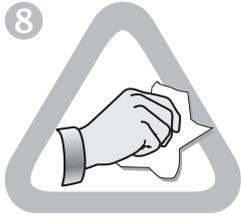
Clean the surfaces of the joint with the impregnated cleaning cloth to remove dirt and grease, etc. Ensure no residual fibres from the cloth remain on the joint area.
