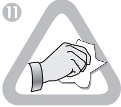
Align the join and wipe clean any excess adhesive from the join area. Ensure that the PTFE strip is in place between the join and the band to stop the adhesive sticking to the band.
