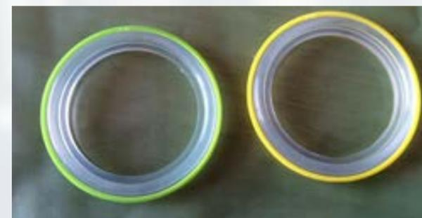
Fully coloured EPDM gaskets are available, however, simply being coloured means no carbon black is present in the EPDM. Carbon black is essential to EPDM to give good mechanical properties, therefore removing carbon black from the material will compromise the properties, and hence performance, leading to problems with intrusion and the need to re-torque at regular intervals.
