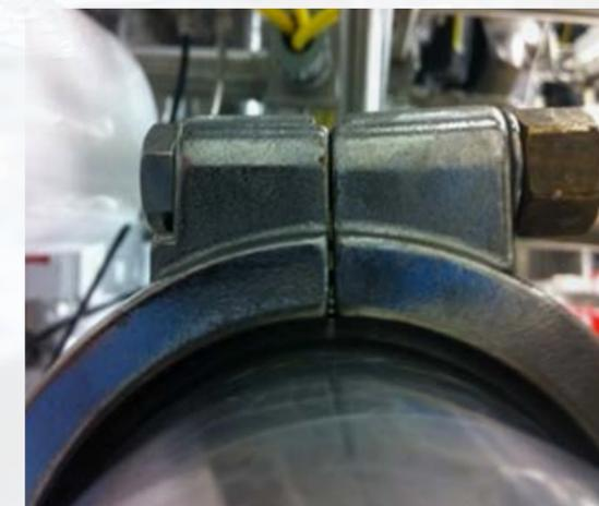
As the picture above shows, the bolt is now bent and will need replacing. Additionally, at such loads it is likely the ferrule will be damaged, and may also need to be replaced.
