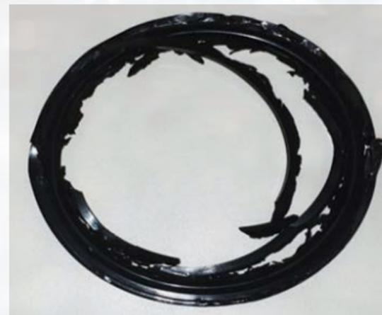
The picture above shows damage around the entire seal and is a direct consequence of applying too much force on the seal by over torquing.
