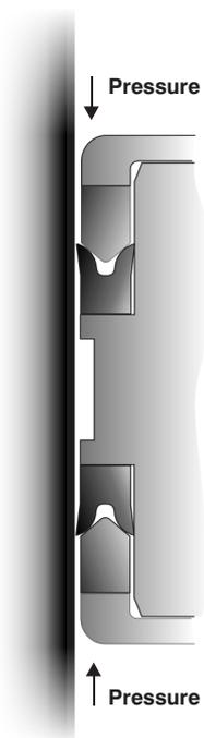
Push U-ring to bottom of housing with its lips facing positive pressure. Insert header ring so its domed face fits snugly between the lips of the U-ring. Ensure lips of U-ring do not turn or are otherwise damaged during assembly.
