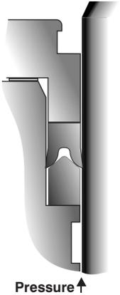
If additional compression is needed to overcome leakage, remove some spacers.
